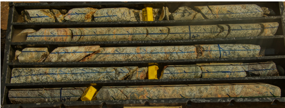
Figure 5. Diamond drill core from hole MDD 006 (metallurgical DD hole) containing potential REE mineralisation from visual inspection (pinkish coral colour) from approximately 41m to 45m down hole
