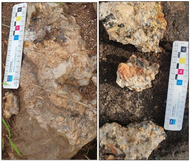
Figure 34: Pegmatitic samples from Machinga South anomaly with radioactive minerals Source: CSA Global (2023)
